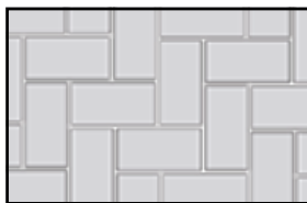
Patrón espina de pez a 90° Pattern at 90° perpendicular to the pass TERANA® SIX acqua joint 20x10x8cm
